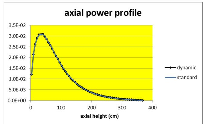
Figure 1: Axial power distribution for central fuel pin for dynamic and standard method
